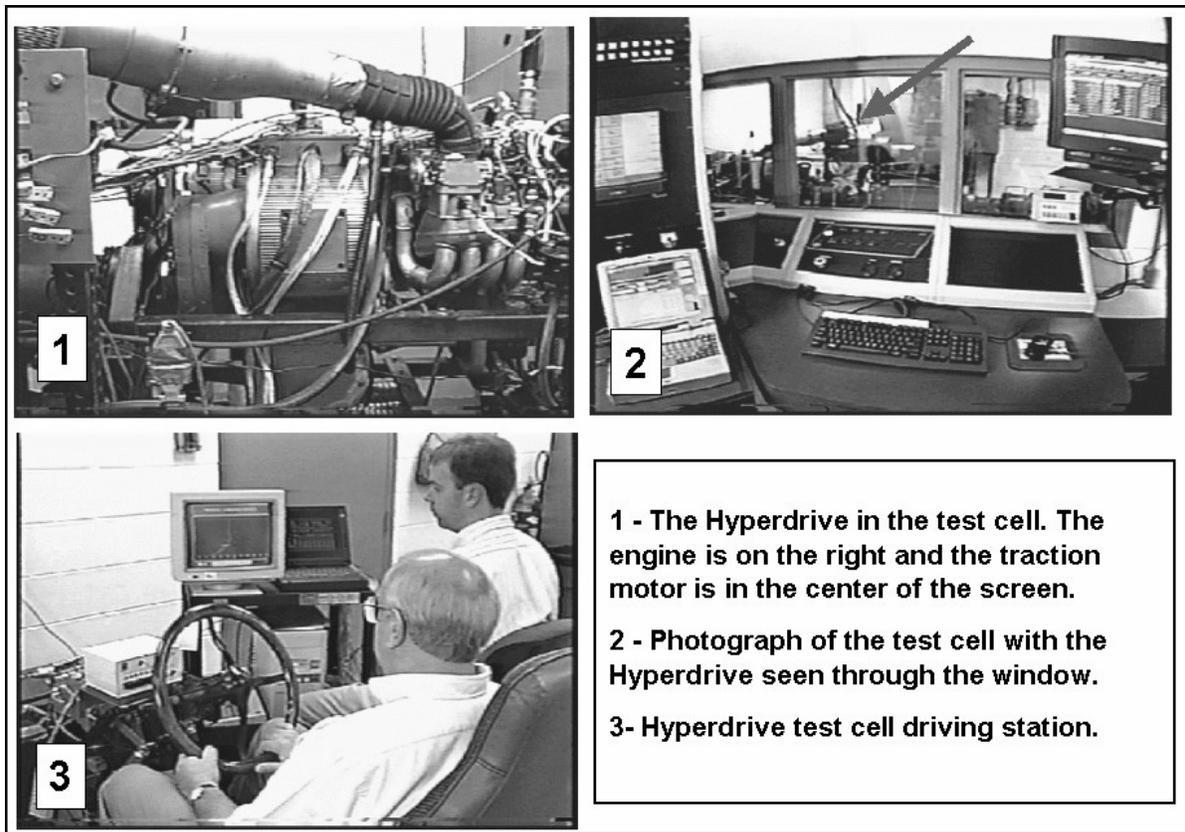
Fig. 3. Hyperdrive in the dynamometer test cell
