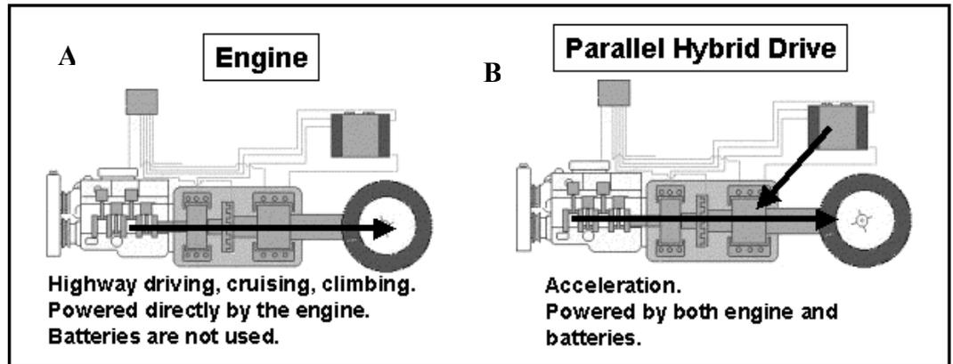
Fig. 5. Typical Hyperdrive operation in highway driving.
