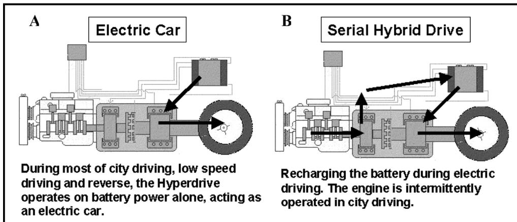
Fig. 4. Typical Hyperdrive operation in city driving.
